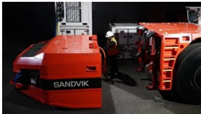
Figure 2 - Sandvik TH550B heavy duty vehicles battery swapping and automated charging
