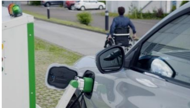
Figure 1 - Ford robotic charging demonstrator
